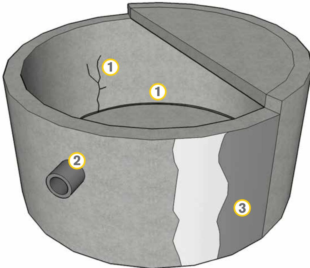
1. Use the Krystol Leak Repair System to treat leaking cracks and joints. Refer to Application Instruction 5.12 — Waterproofing Cracks, Holes and Joints.
