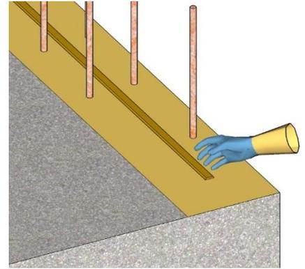
**IMPORTANT:** Contact with water will result in premature swelling of the strip. Protect the installed Krytonite from water until concrete is poured. If premature swelling occurs, Krytonite must be dried to restore its original dimensions before pouring concrete.
