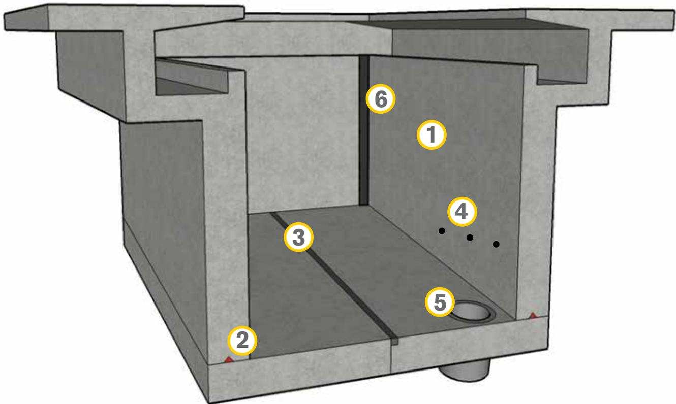
1. Add Krystol Internal Membrane (KIM) to the concrete mix in the base slab and walls to ensure water is contained and not contaminated from outside sources. Refer to Application Instructions 1.11 to 1.15 — Use of KIM Admixture.
