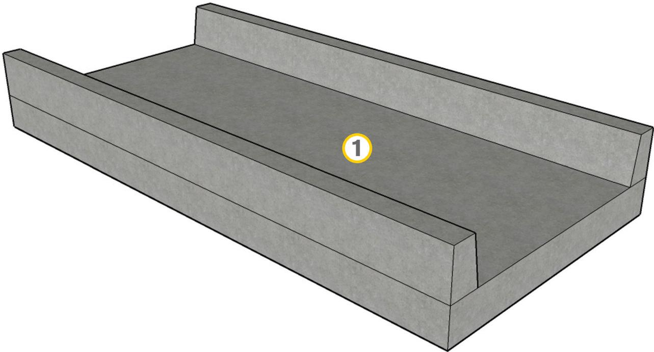
1. Add Krystol Internal Membrane (KIM) to the concrete mix in the bridge deck to protect the deck from de-icing salts. Refer to Application Instructions 1.11 to 1.15 — Use of KIM Admixture.
