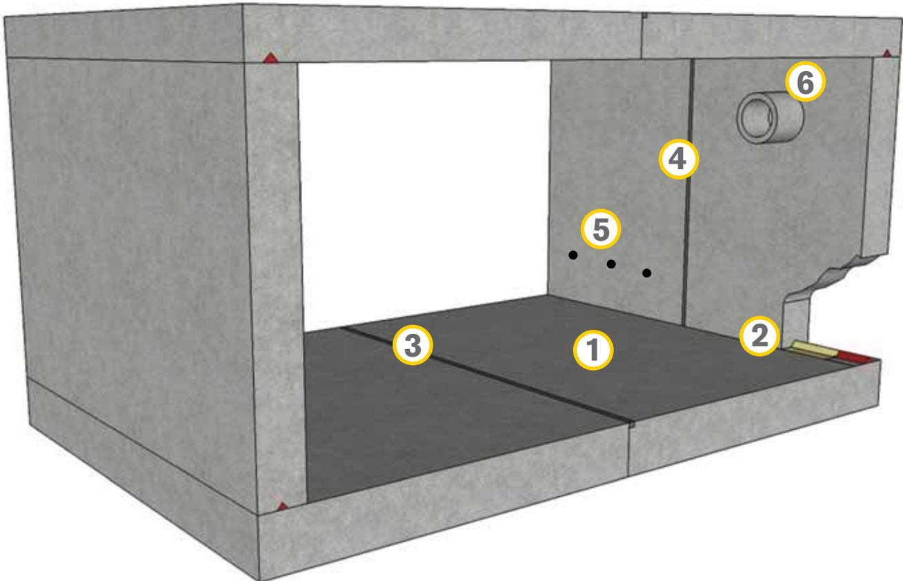
1. Add Krytol Internal Membrane (KIM) to the concrete mix to protect the slab and walls from water ingress and other contaminants. Refer to Application Instruction 1.11 to 1.15 — Use of KIM Admixture.
