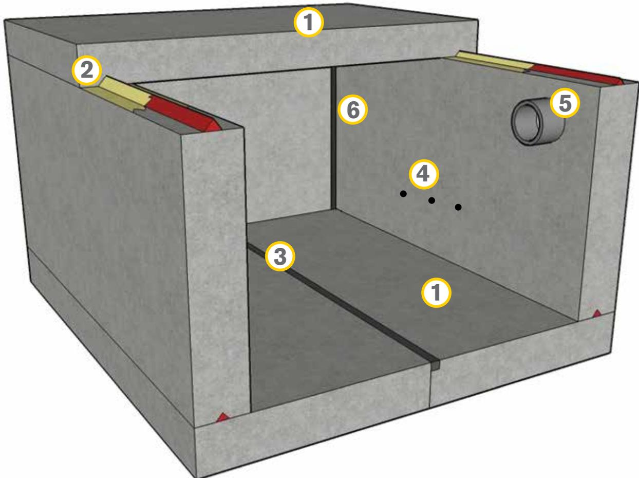
1. Add Krystol Internal Membrane (KIM) to the concrete mix to ensure water is contained and not contaminated from outside sources. Refer to Application Instruction 1.11 to 1.15 — Use of KIM Admixture.
