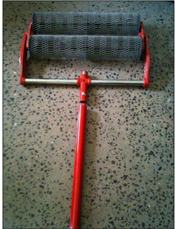
**A pass or two with a roller-bug may help create surface paste and embed fibers**
