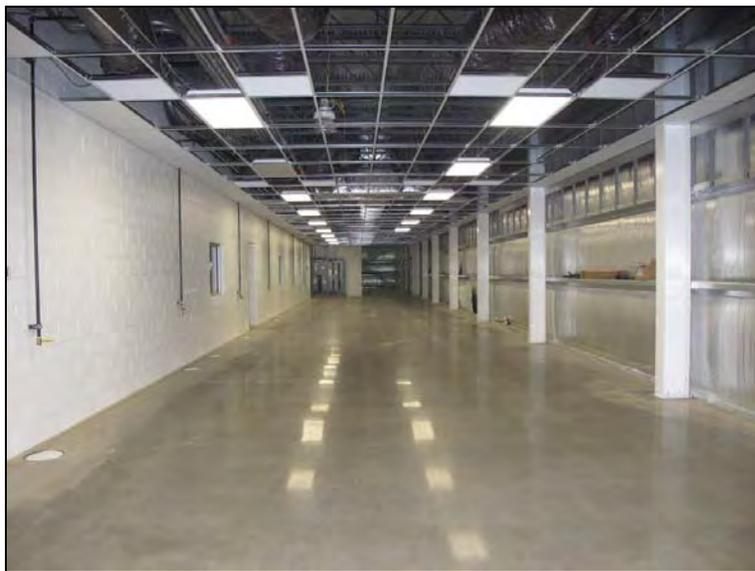
**Highly-reflective deep aggregate grind floor**
