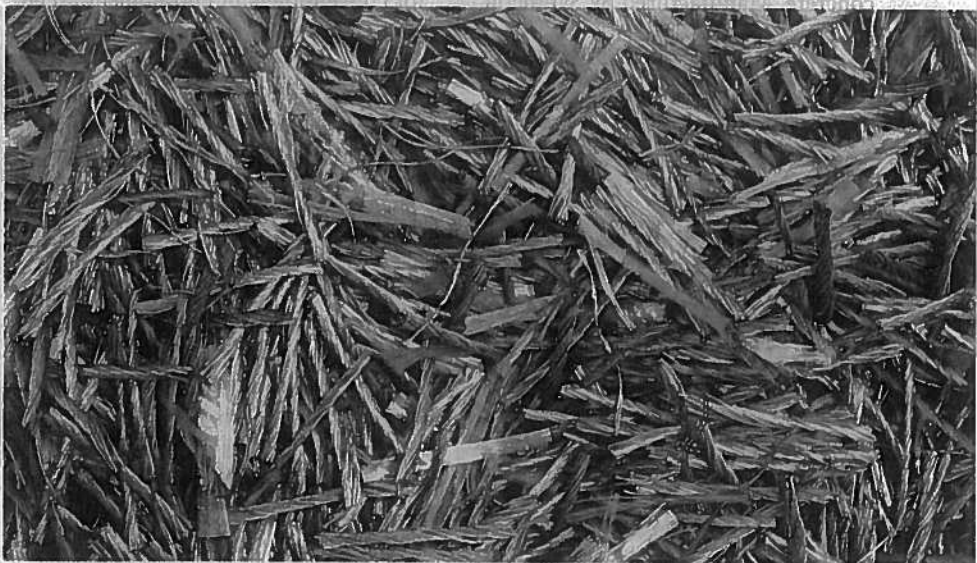
Configuration of macro-synthetic fiber allows reinforcement to be used in high dosages. With earlier micro-synthetic fibers, high dosages made mixing, placing, and finishing difficult. PHOTO: FORTA CORP.
