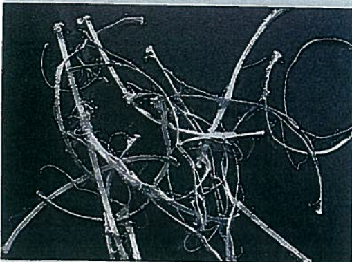
Synthetic structural fiber before mixing is shown (top), and self-fibrillating of the fiber after mixing (bottom).
