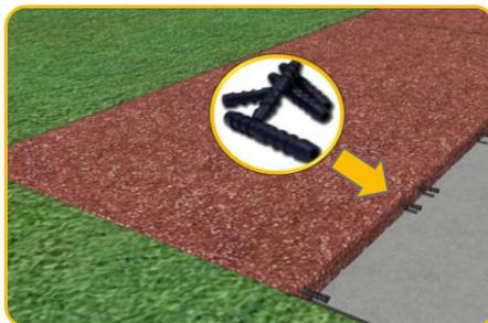
Install the second row offsetting to the first row of half plate. Continue offsetting the other rows to complete the surface
