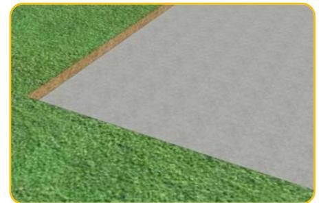
Apply the glue on the concrete surface with a notched trowel of 3 mm
