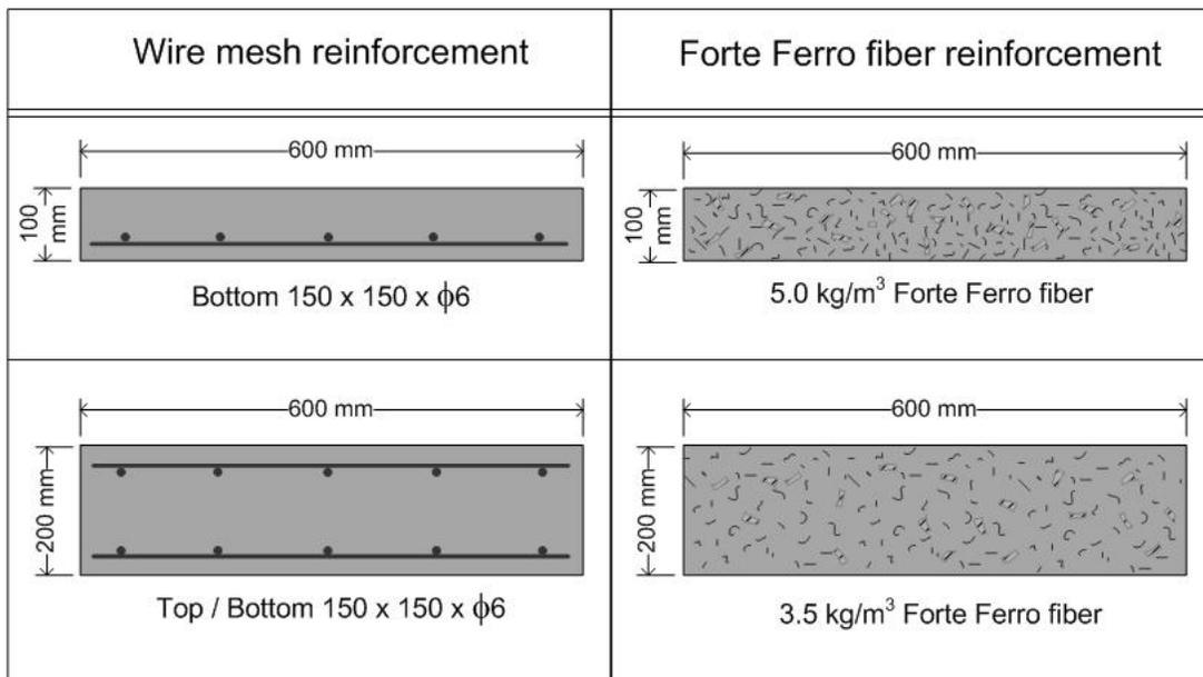
**Figure 3:** Specimen details
