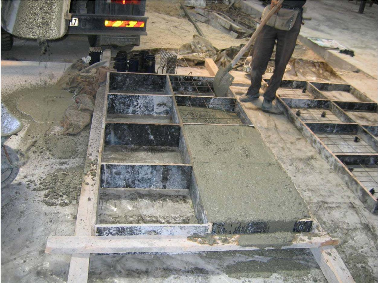
**Figure 2:** Production of concrete plate specimens
