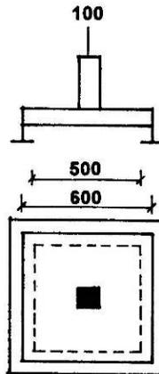
The plate shall be produced from a sprayed panel by levelling the panel at a thickness of 100mm - 0/+10mm, immediately after spraying. The sloped edges of the panel shall be sawn off when the plate is prepared in the laboratory. The prepared plate shall be stored in water for a minimum of 3 days immediately before testing and kept moist during testing.
