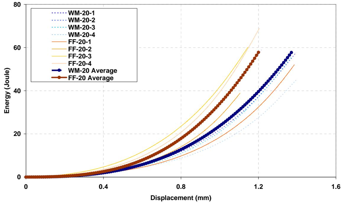
(c) Energy-Displacement relationships until first crack (200mm concrete plates)
