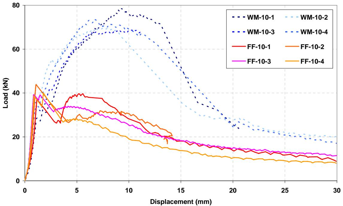
(b) Load-Displacement relationships at ultimate loading (100mm concrete plates)
