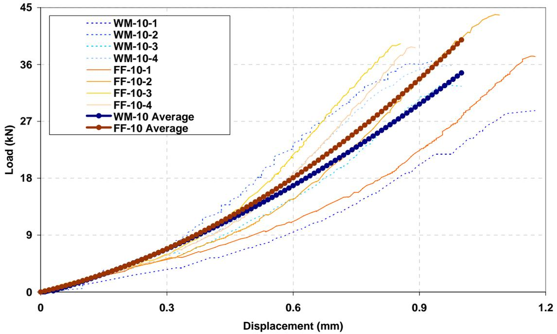
(a) Load-Displacement relationships until first crack (100mm concrete plates)
