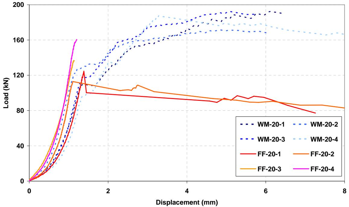
(d) Load-Displacement relationships at ultimate loading (200mm concrete plates)
