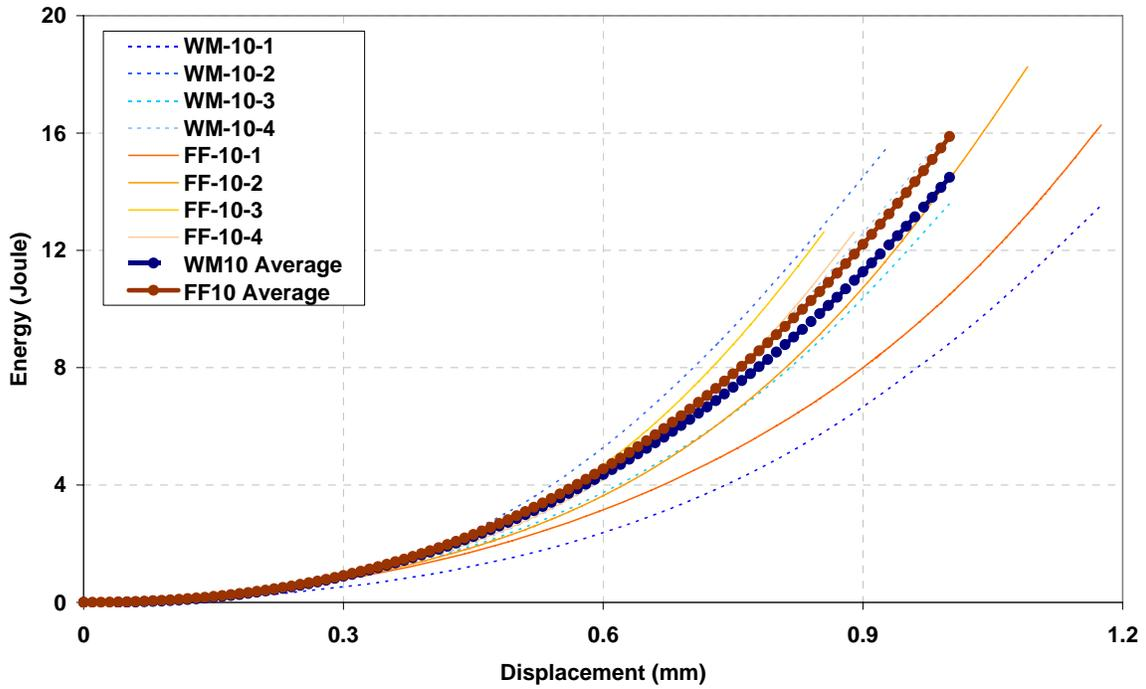
(a) Energy-Displacement relationships until first crack (100mm concrete plates)
