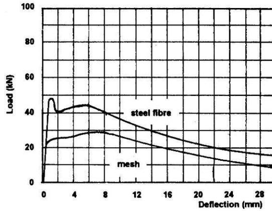
Figure 10.4.3: Example of energy-deformation curves
