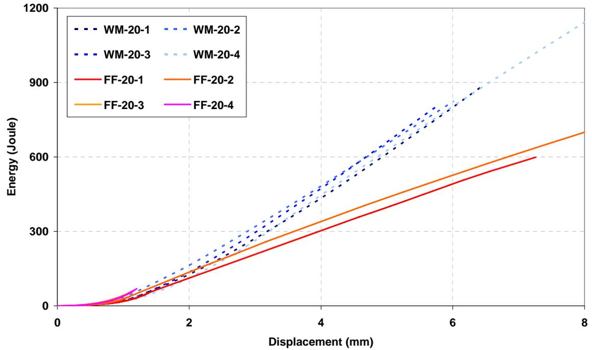
(d) Energy-Displacement relationships at ultimate loading (200mm concrete plates)
