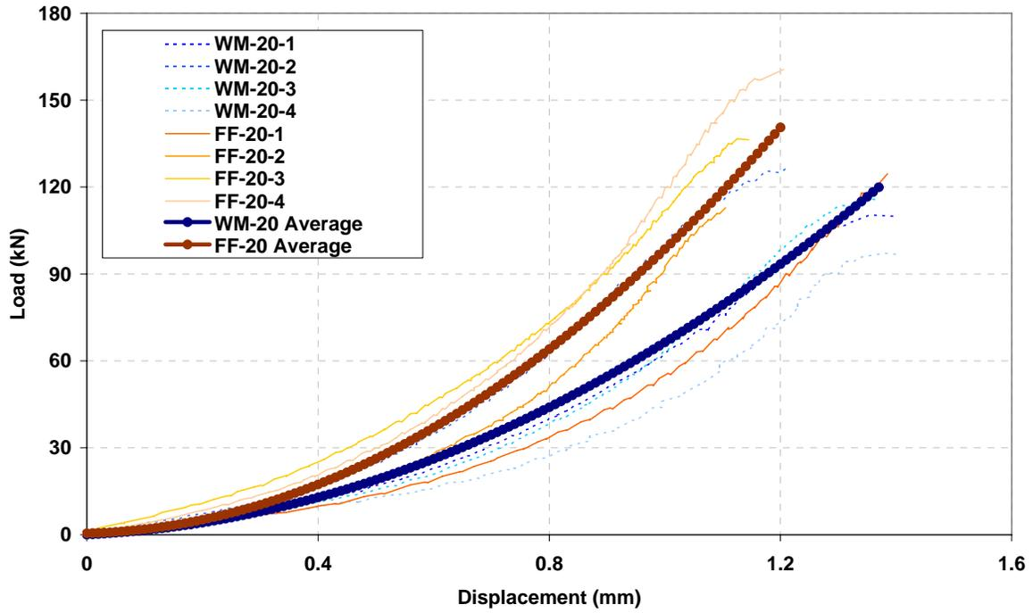
(c) Load-Displacement relationships until first crack (200mm concrete plates)
