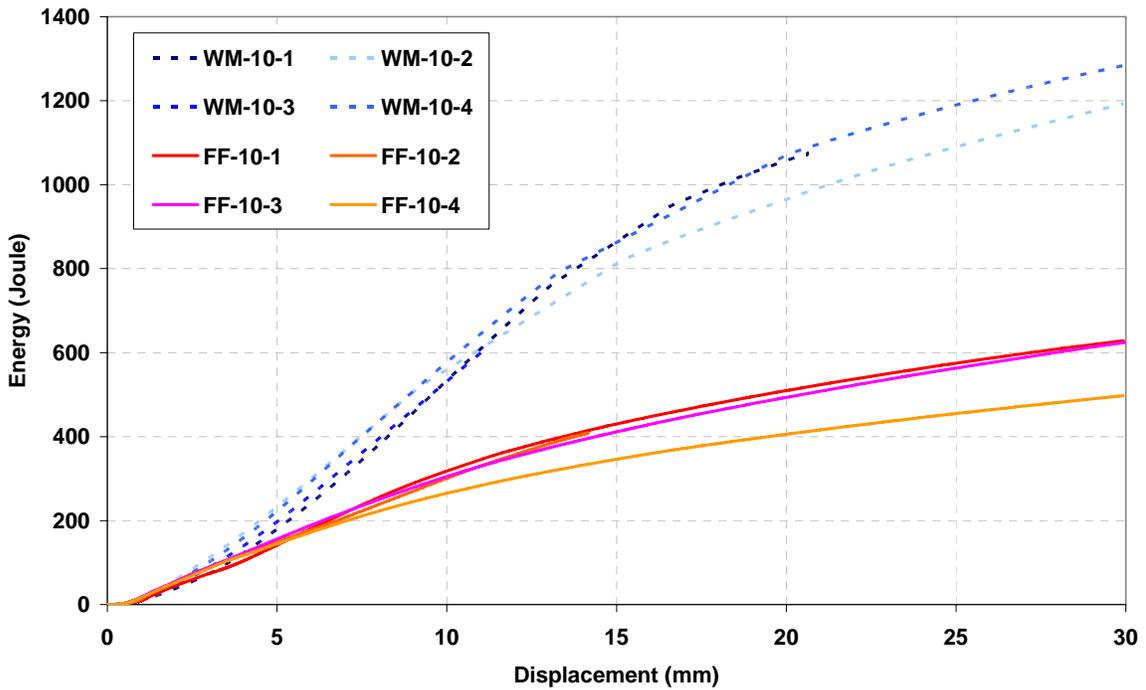
(b) Energy-Displacement relationships at ultimate loading (100mm concrete plates)
